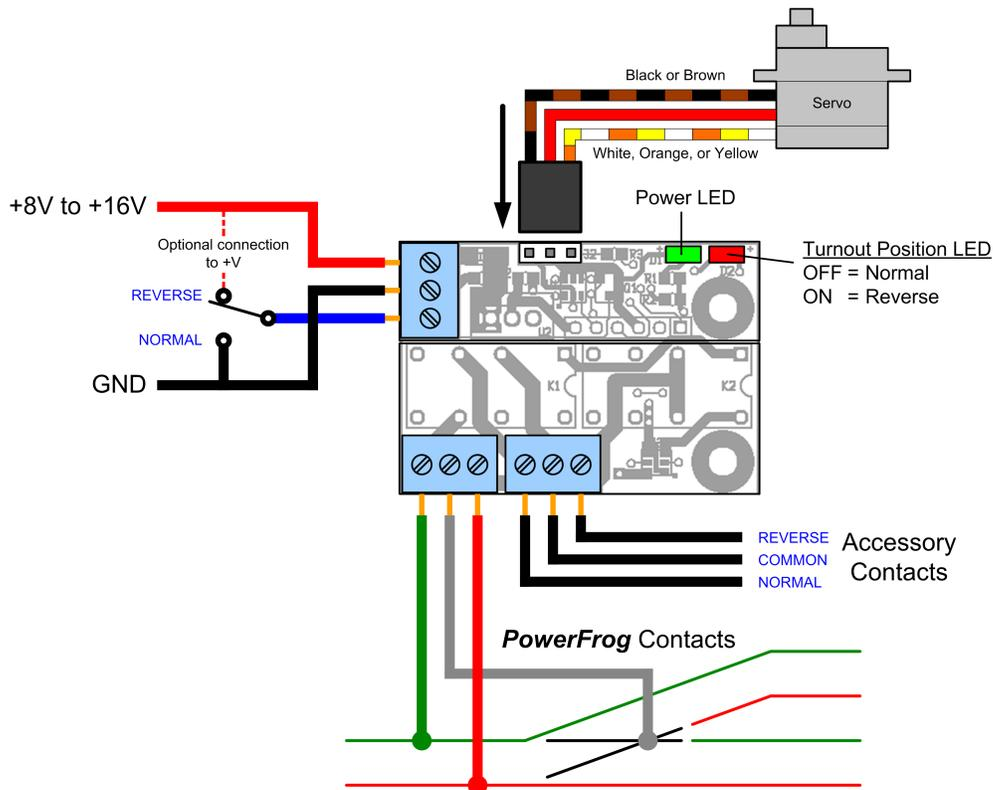
*Typical wiring for a MRServo-3. MRServo-1 boards will only have the upper half of the board (power, control, and servo connections), and MRServo-2 boards will have an additional set of accessory contacts (with the same pinout as the first) in place of the PowerFrog contacts.*
